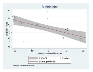
The bubble plot is a scatterplot of effect sizes and covariate values. Each study is represented by a circle with the size of the circle proportional to the effect-size precision,  $1/\hat{\sigma}_j^2$ . The fitted line (predicted log risk-ratios) is also plotted on the graph.
